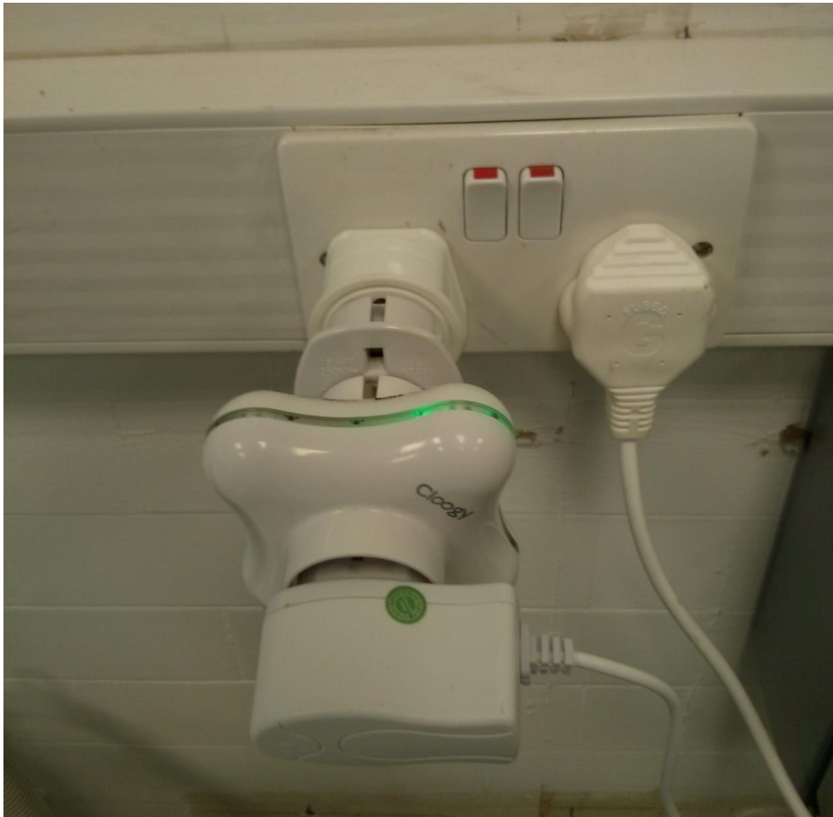
Figure 8 - Example of usage of UK/EU adapters for Cloogy power plug
