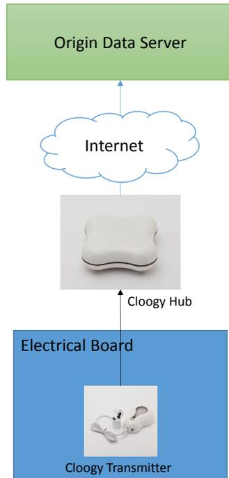
Figure 2 - Basic Monitoring Module Layout
