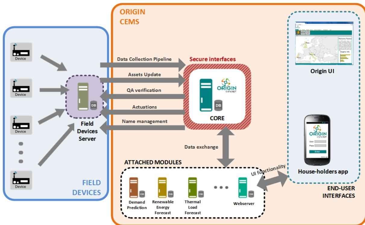
Figure 1 - ORIGIN platform high-level architecture
